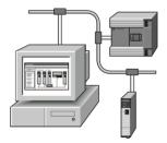
graphical representation of your network configuration and configure the parameters that define your network. RSNetWorx for ControlNet software schedules network components. The software automatically calculates network bandwidth for the entire network, as well as the bandwidth used by each network component. You must have RSNetWorx software to configure and schedule the ControlNet networks in your PLC-5 programmable controller system.
